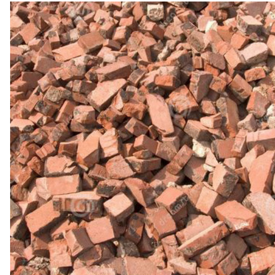
Typical reclaimed aggregates
